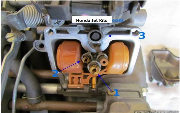
To the far left is the Pilot Screw. The Main Jet is in the center and is screwed in the jet holder. Remove pilot jet and main jet using a flat screw driver.
